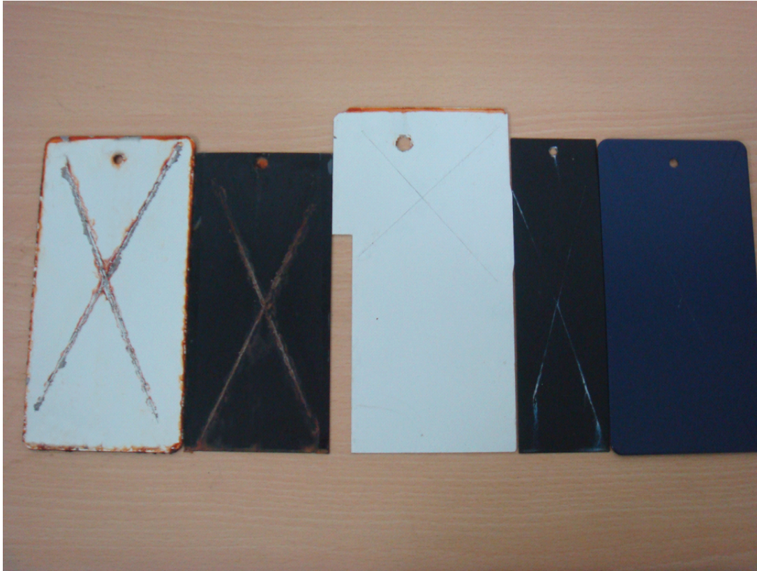
cold plate painting cold plate electrophoresis galvanized plate/coating galvanized plate/ spray Al plate powder spray
